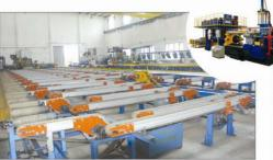
3600 Tons large-size extrusion producing line
